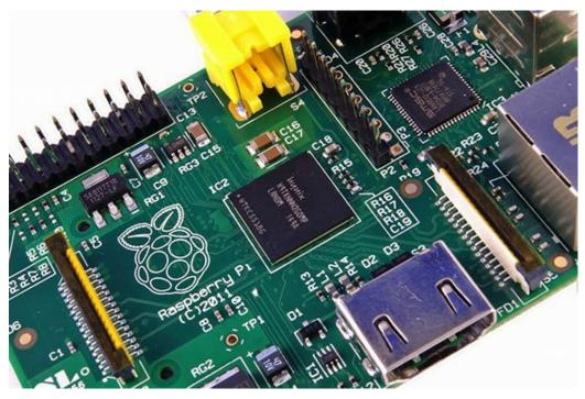
Developed by Acorn Computers back in the late 1980s, the ARM architecture is a relatively uncommon sight in the desktop world. Where it excels, however, is in mobile devices: the phone in your pocket almost certainly has at least one ARM-based processing core hidden away inside. Its combination of a simple reduced instruction set (RISC) architecture and low power draw make it the perfect choice over desktop chips with high power demands and complex instruction set (CISC) architectures.
