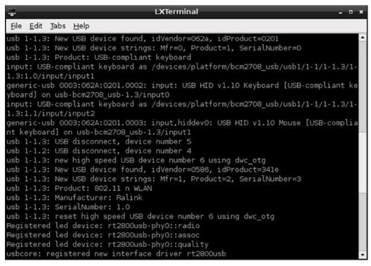
The important part of this output is the line that reads Manufacturer. In the case of the example Zyxel NWD2105, this reads Ralink, which is the company that makes the actual chip found inside Zyxel USB wireless adapter. It's this company's firmware that must be installed for the wireless adapter to work.
