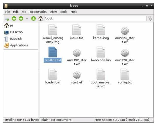
In a Linux-based desktop or laptop, these options are normally passed to the kernel by a tool known as a bootloader, which has its own configuration file. On the Pi, the options are simply entered directly into cmdline.txt to be read by the Pi at startup.
