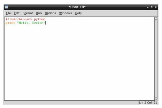
Before you run your program, save it as helloworld.py using the File menu. If you're using IDLE, the file will be given the extension .py automatically. If you're using a text editor, be sure to type .py at the end of the filename (not .txt) when you save it. This extension indicates that the file contains Python code—although Python is clever enough to run the program even if it's saved with a different file extension.
