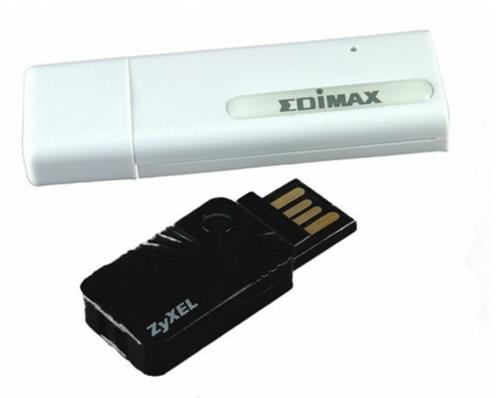
Using such a device, the Pi can connect to a wide range of wireless networks, including those running on the latest 802.11n high-speed standard. Before purchasing a USB wireless adapter, check the following:
