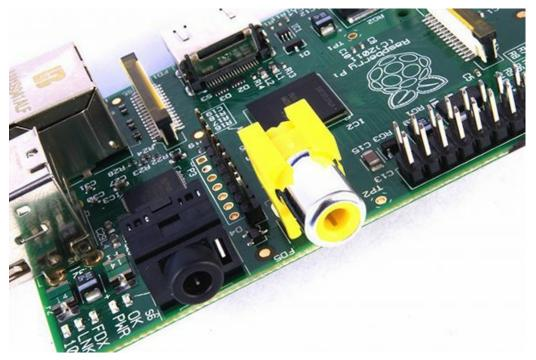
When no other display device is available, a composite video connection will get you started with the Pi. The quality, however, isn't great. Composite video connections are significantly more prone to interference, lack clarity and run at a limited resolution, meaning that you can fit fewer icons and lines of text on the screen at once.
