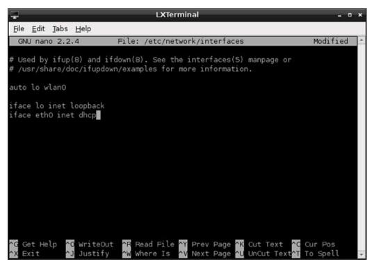
When you've finished editing the file, press CTRL + O to save it, and then press CTRL + X to leave nano and return to the terminal. To use your new network settings, restart the networking service by typing the following:
