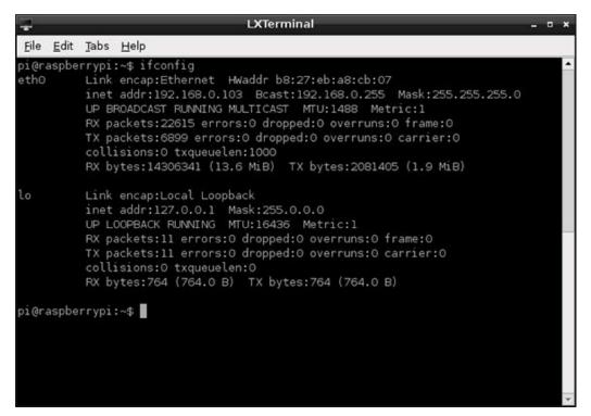
The output of ifconfig is split into the following sections:
