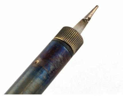
This process of tinning the tip protects it against damage and ensures that it will efficiently transfer heat onto the surfaces to be soldered. Failure to properly tin the iron's tip is one of the most common causes of bad solder joints. You may need to repeat this process more than once if you're soldering a lot of connections, and you'll need to do it again at the end of the soldering session. In general, if the tip of the soldering iron loses its shiny coating, repeat the tinning process.
