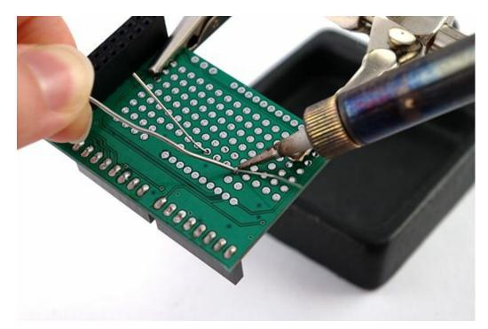
**4.** As the solder flows, you'll see it drawn down into the hole in the board. This is an indication that the area is hot enough for a good solder join. If the solder floats, it indicates that the area is not yet hot enough.
