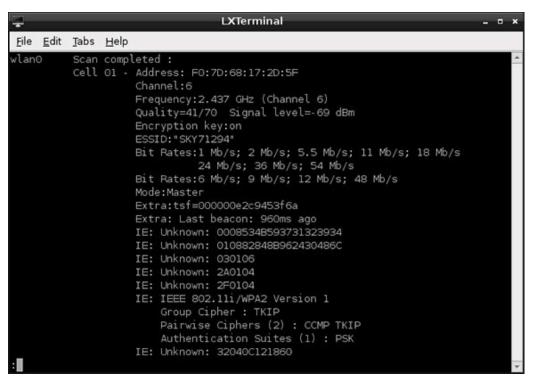
You can check the current status of the network using the iwconfig command. Like ifconfig, the iwconfig command allows you to check the status of a network interface and issue configuration commands. Unlike ifconfig, however, iwconfig is specifically designed for wireless networks and includes specific features for this. Type the command name at the terminal as follows:
