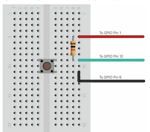
Figure 12-5: The example breadboard layout for a simple push-button input
